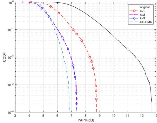
Fig. 1. PAPR reduction performance of  $k$ -MQP and UC-CMA
