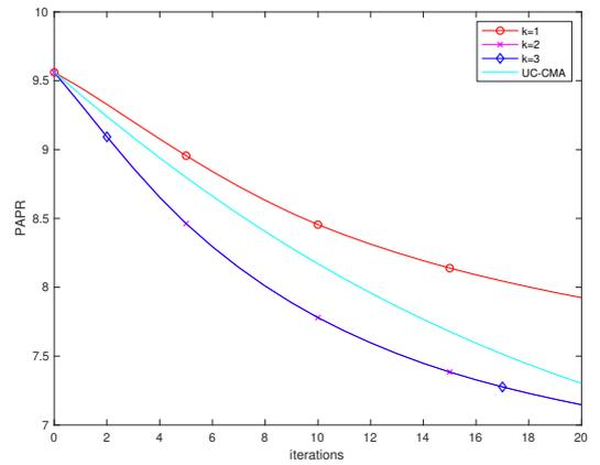
Fig. 3. comparison of average PAPR values versus outer-loop iteration numbers for  $k$ -MQP and UC-CMA
