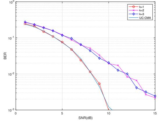
Fig. 2. BER performance comparison of  $k$ -MQP and UC-CMA
